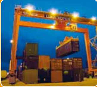
Rubber tired gantry crane, RTG.
