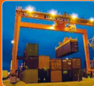
1- Rubber tired gantry crane, RTG.
